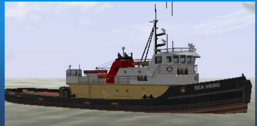
Mono-screw conventional tug- pusher with flanking rudders, 31 t.
